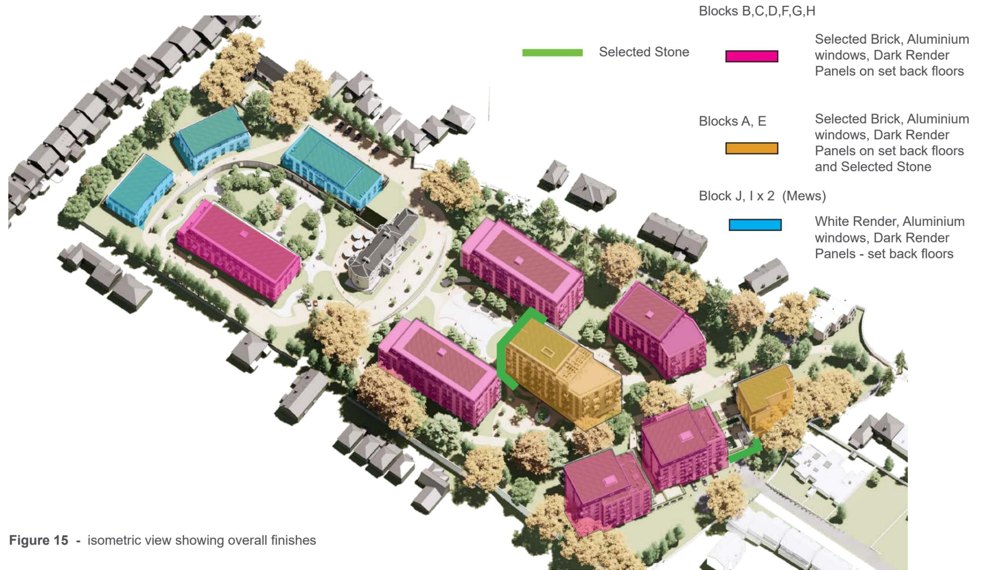
Figure 15 - isometric view showing overall finishes
