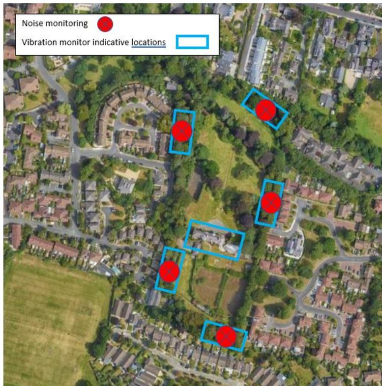
**Figure 5** Construction Monitoring Locations
