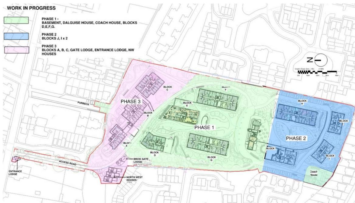
Figure 5.1: Illustrative Plan showing proposed construction phasing.
